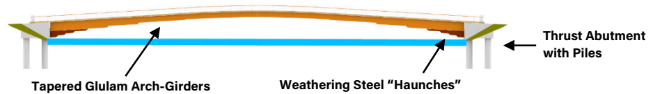
Figure 8 - Sketch showing the low profile of the bridge in relation to the embankments. Credit: StructureCraft
